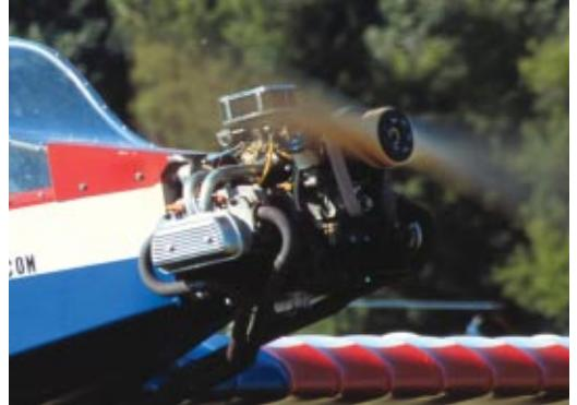
Also, [your] recommendation of installing a reduction drive with a jack-shaft to cancel resonance is totally wrong. Molt Taylor and many others have found that a long shaft will amplify resonance between an engine and the prop.
